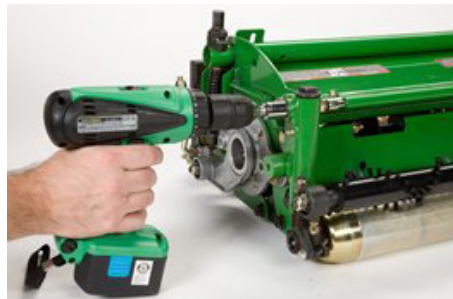
Adjustment with cordless drill
