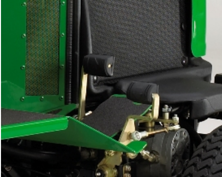
Dual-pedal for forward and reverse
