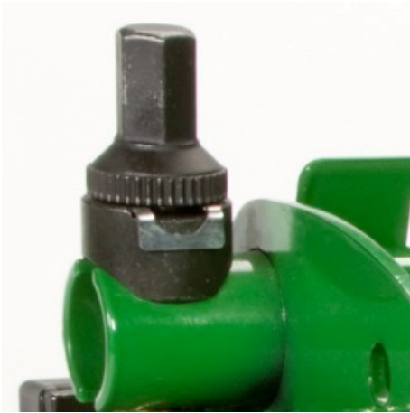
Close-up of reel-to-bedknife adjustment
